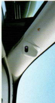
Fatigue Monitoring System
